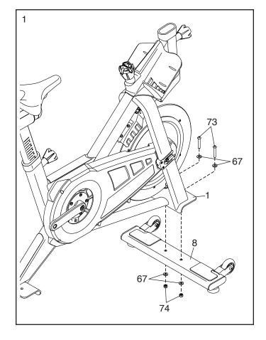
2. Attach the Rear Stabilizer (7) to the Frame (1) with two M10 x 50mm Bolts (73), four M10 Washers (67), and two M10 Locknuts (74).
