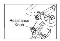
To stop the flywheel, push the resistance knob downward. The flywheel should quickly come to a complete stop.
